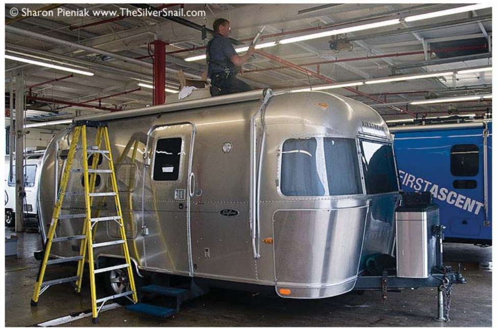
AT JACKSON CENTER - Worker prepares to seal roof seams with caulk.
